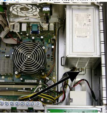
Figure 5-44 Removing the power supply, release lever
